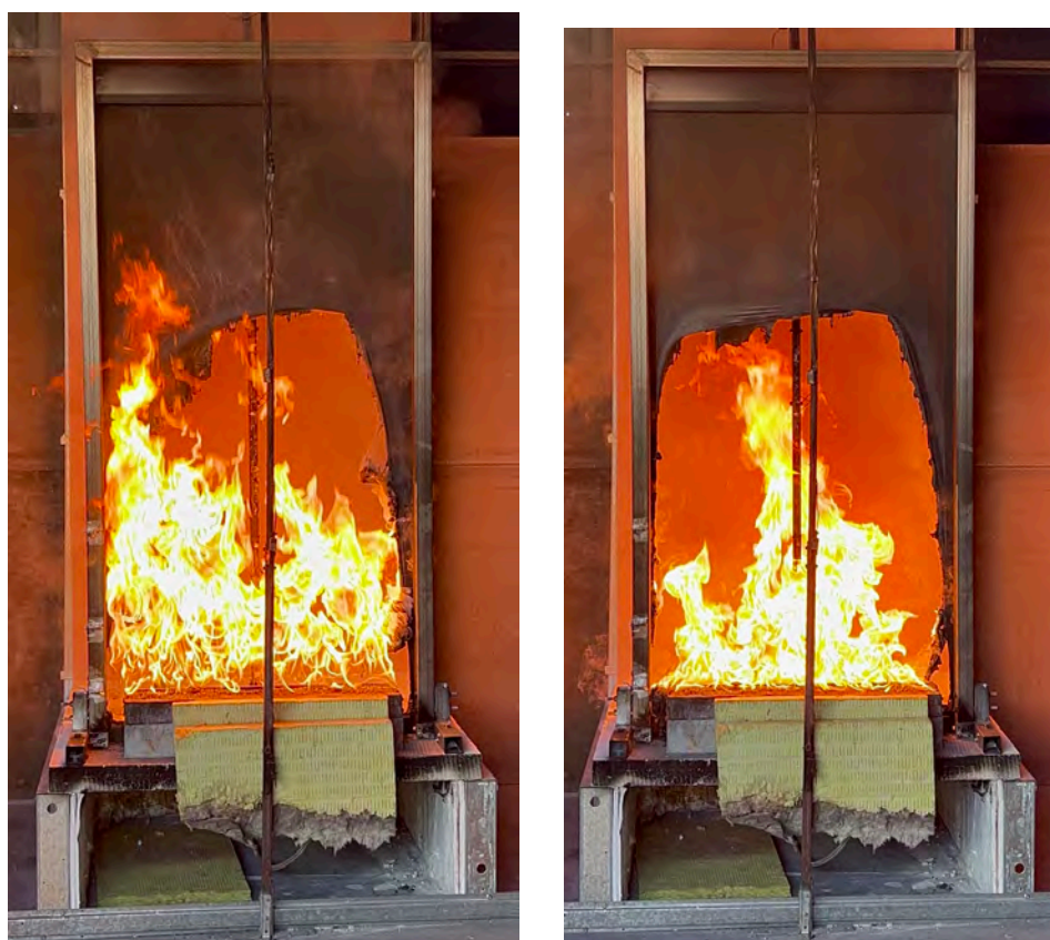
FIGURE 11: MATERIAL REACTION DURING DIRECT FLAME IMPACT
