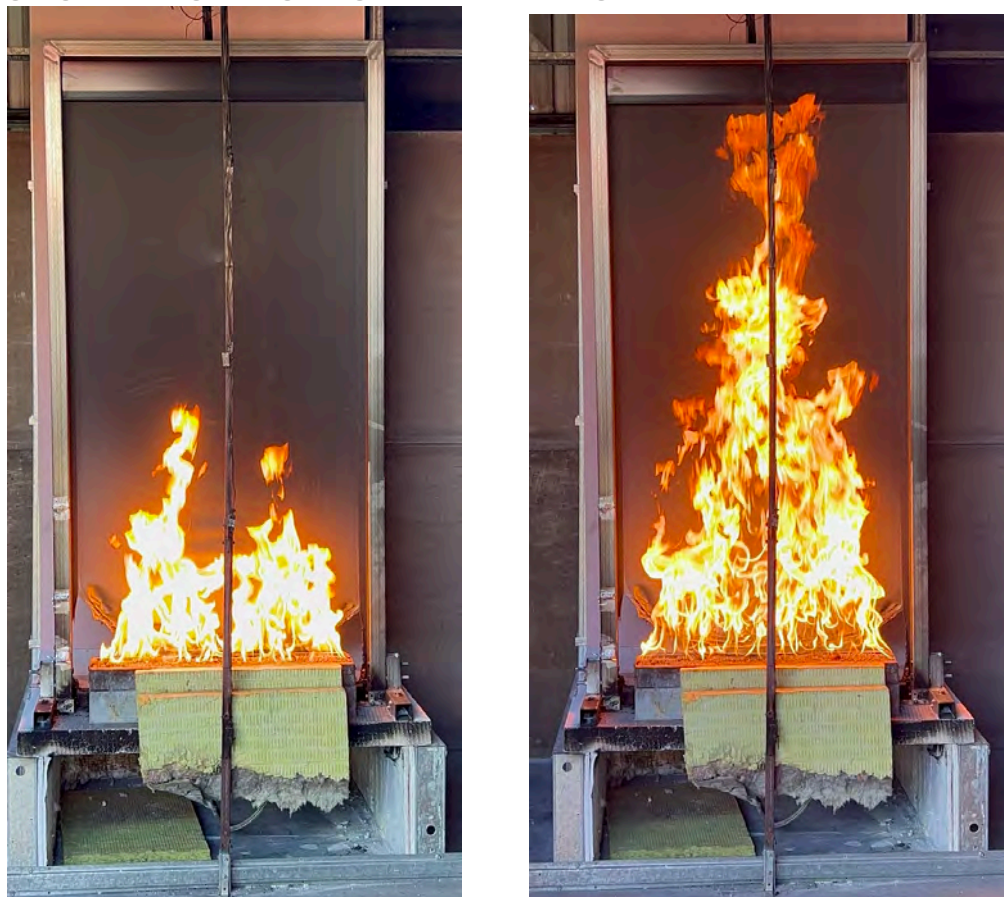
FIGURE 10: SPECIMEN AT START OF TEST AND PEAK FIRE SIZE
