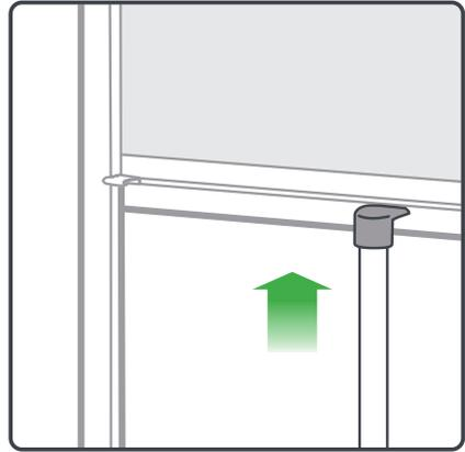
When operating the blind using a pull stick, the pull stick should only be placed in the centre of the bottom bar to push/pull the blind up or down. Pressure should only be applied on the lip of the bottom bar.
